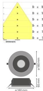
**Scheda tecnica Ledvance Downlight LED Performance DN155 14W 1600lm 65D - 840 Bianco Freddo | 180mm - IP54 - Dali Dimmerabile**
